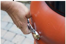
Use adjustable wrench to tighten overflow valve.
