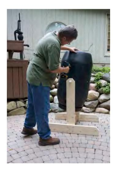
Drill 1/2" vent holes around top & bottom.
