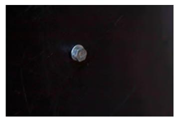
To assemble the rake system start by drilling a hole with the 13/64" drill bit. Drill the first hole at the center of the drum just below the center pole, so the center pole does not obstruct the rake system. Then drill two additional holes 5" away on each side. Use nuts and lock washers to tighten. Then use hacksaw to cut the extra.
